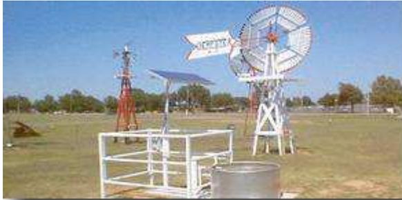
There are still thousands of windmill water pumping units standing in the Western US. Regrettably, many are inoperable. These pumpers were very valuable for remote (off grid) sites, with the proper minimum wind conditions, when manpower was plentiful and cheap. Windmills, though potentially long lasting, need dedicated maintenance. The down hole leathers require inspection and high
